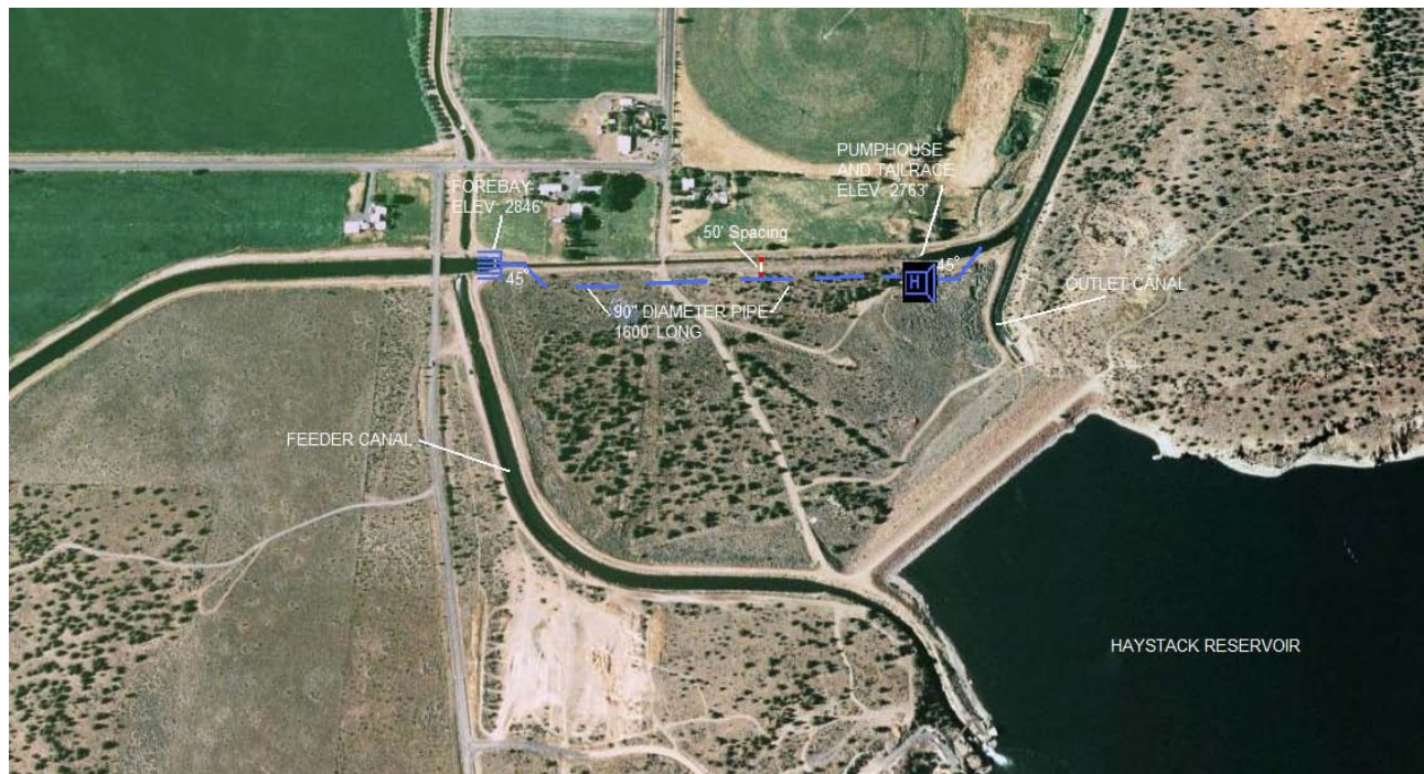
Figure 3: Haystack Reservoir Bypass Canal Alternative
