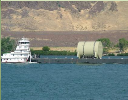
A Navy submarine reactor compartment on the Columbia River, heading to Hanford.
